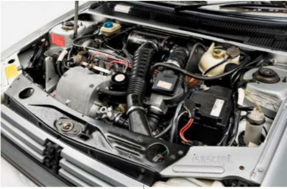
A quirk of both the 1.6 (here) and the 1.9 is jerky acceleration. The Bosch K-Jetronic injection system used a switch rather than a throttle position sensor
