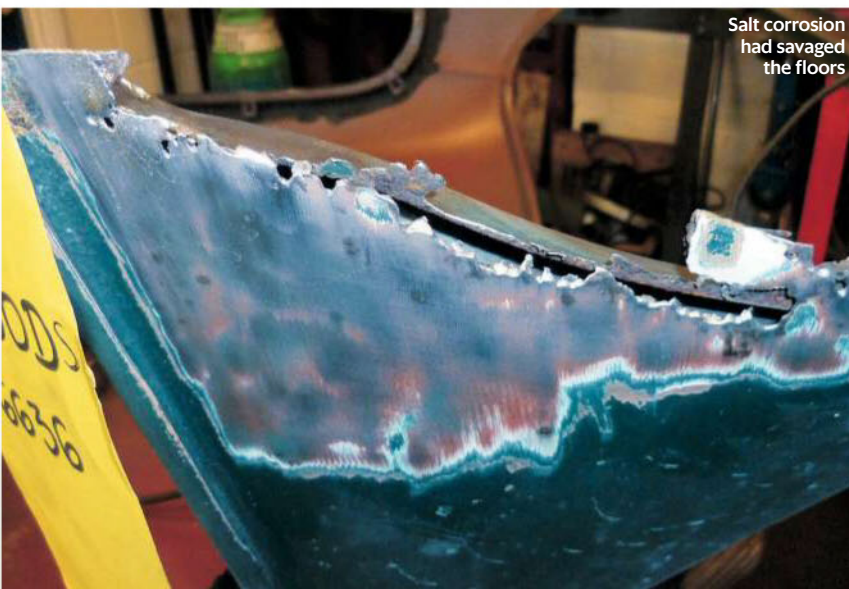
Rust-ravaged bulkhead replaced with a MkIII panel
