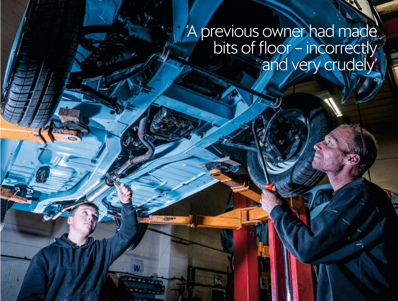
Salt corrosion had savaged the floors
