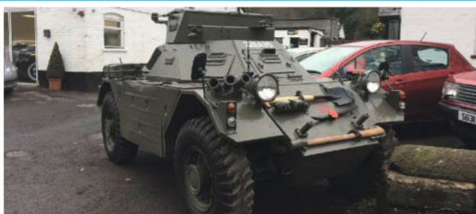
1962 Daimler Ferret Scout Car. 4 wheel drive with Rolls Royce 4.2 litre, 6 cylinder engine. Wilson pre-selector gearbox, 5 forward gears and 5 reverse gears, each capable of doing 59 miles per hour. Full spec including de-activated smoke grenade launchers (3 either side), periscope, shovels, axe and gerry cans. Part of private collection for last 17 years, unregistered, last used in circa 1992 with the Royal Hussars on the Rhine. Very unusual and interesting vehicle, we are told that 31 countries still use these..... £18,950
